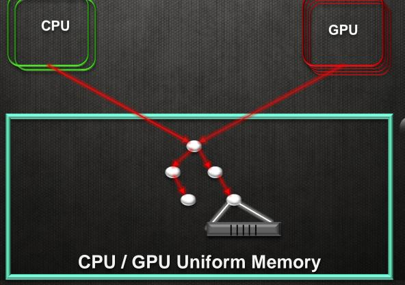
CPU can pass a pointer to entire data structure since the GPU can now follow embedded links
